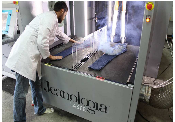
1- Suction and filter centralized system with individual regulatory and control system by machine, optimizing costs and performance.
